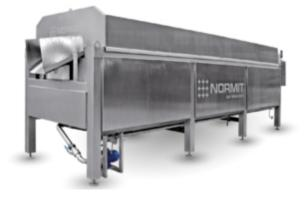
Individual Design Engineering Continuous screw blancher is designed and manufactured in accordance with the nature of the product, the required performance and customer requirements of the technological process.
